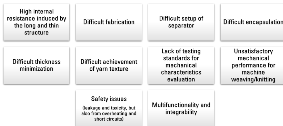
Fig. 2: The technical difficulties encountered by the 1D textile-based batteries for future wearable applications [18]
